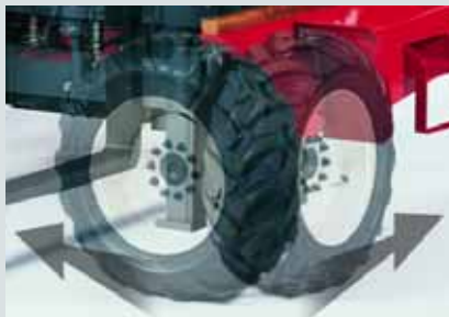
4-way travel is available on a number of machines – ideal when delivering long loads into tight access areas or through doorways.
