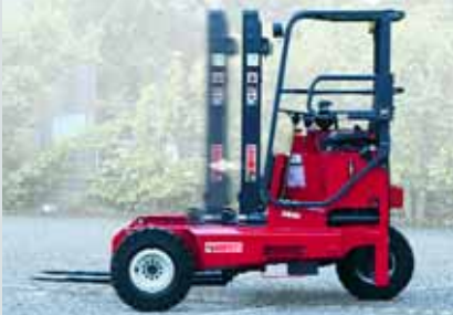
With moving mast models the load is positioned by lateral movement of the mast.
