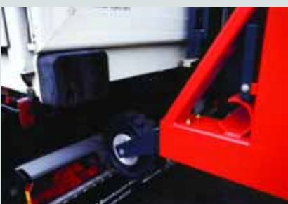
Telescopic legs bring Moffett-Kooi capabilities to trailers with limited overhang behind the rear axle.
