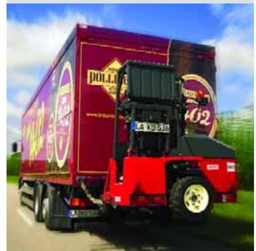
4-way travel is available on a number of machines – ideal when delivering long loads into tight access areas or through doorways.
